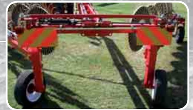
■ Rear drawbar with steering mechanism
