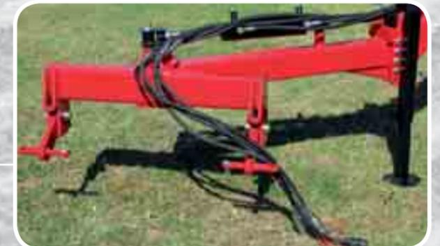
■ 2 point hitch with hydraulic cylinder
