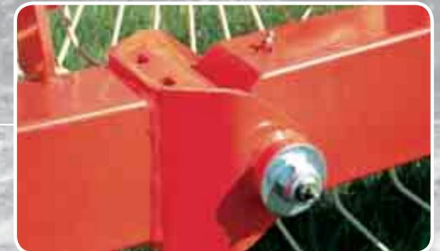
Flex frames on 18-20 models allow greater flexibility over all types of terrain.
