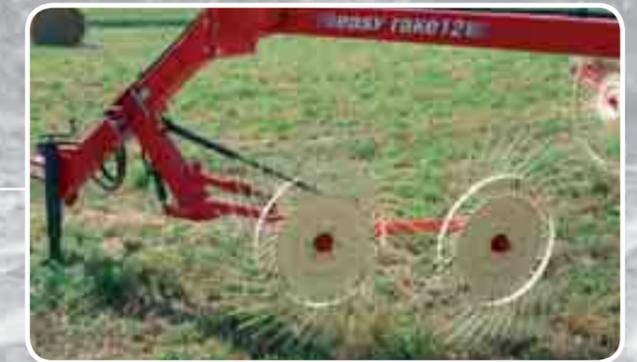
Hydraulically controlled double center kicker wheel
